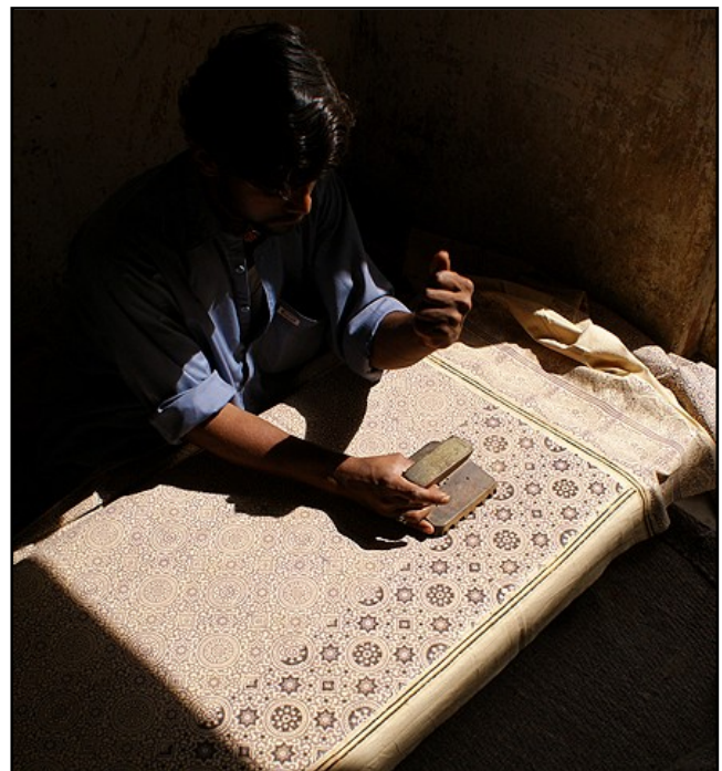
Printer using a traditional block pattern carefully applies dye to the cotton.
